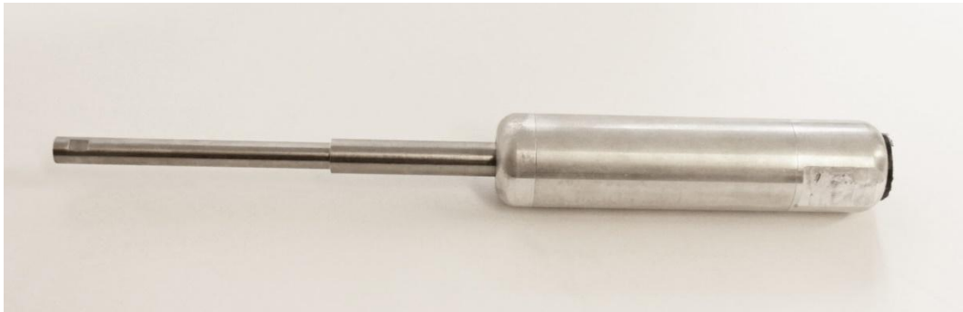
Figure 3: TORS Cement Transducer
